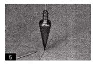
**5**. Drop a plumb bob from the center of the soffit to determine the column's center point on the floor. Mark this point for reference to align the shaft in the proper position,
